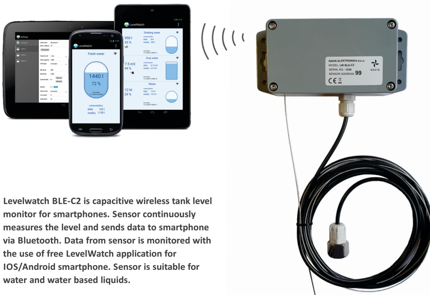
Levelwatch BLE-C2 is capacitive wireless tank level monitor for smartphones. Sensor continuously measures the level and sends data to smartphone via Bluetooth. Data from sensor is monitored with the use of free LevelWatch application for IOS/Android smartphone. Sensor is suitable for water and water based liquids.
