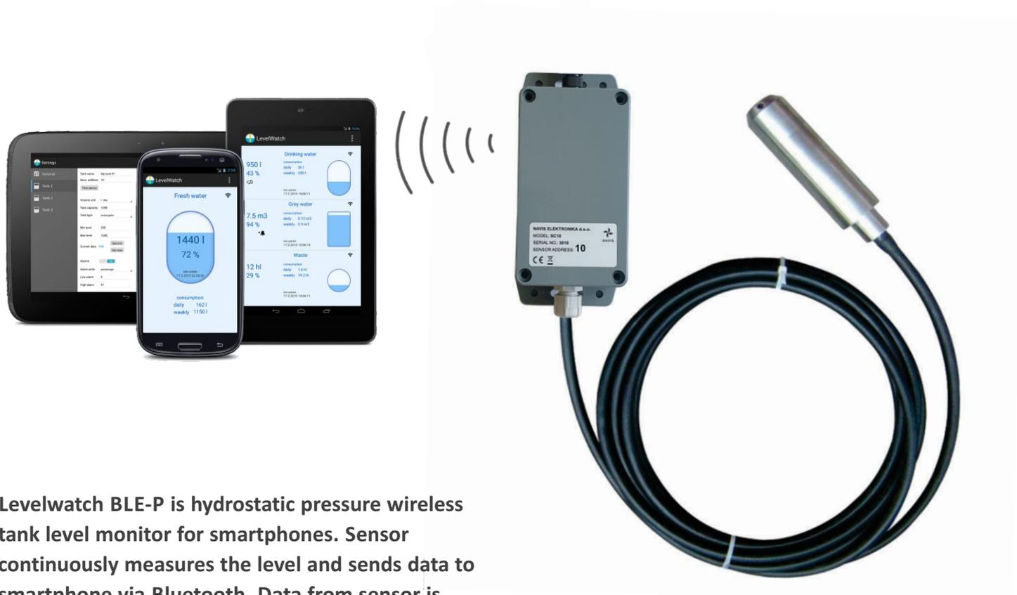
Levelwatch BLE-P is hydrostatic pressure wireless tank level monitor for smartphones. Sensor continuously measures the level and sends data to smartphone via Bluetooth. Data from sensor is monitored with the use of free LevelWatch application for IOS/Android smartphone. Drop-in sensor is suitable for clean liquids.
