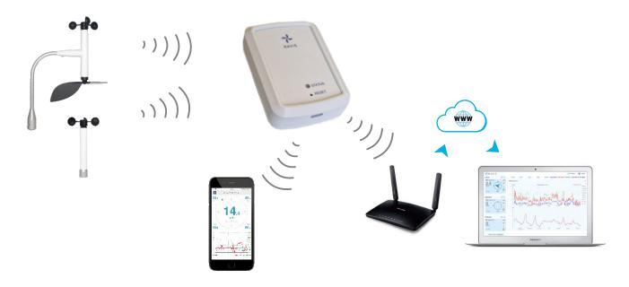
Windy HUB gateway receives data from up to three Navis long-range sensors via radio 868 MHz communication and transmits it via Wi-Fi connection to Navis LiveData web interface.
